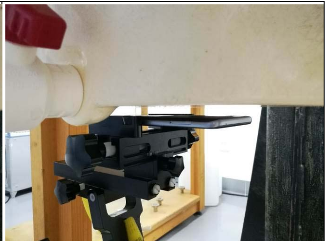
Back Side of EUT with 1.0cm Gap
