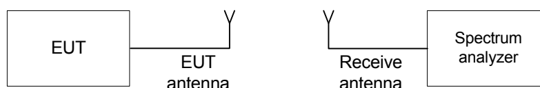
Figure 7.1.1 The 20 dB bandwidth test setup
