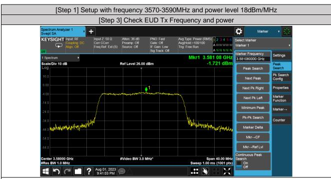
EIRP PSD=-1.721+0.5+5.0+3.01=6.789dBm/MHz, loss of Cable and Splitter is 5.0dB, Antenna gain is 0.5dBi, Array gain is 3.01
