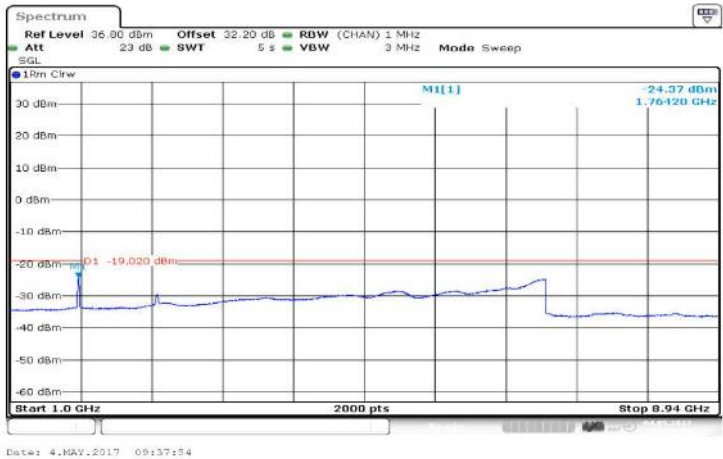
Figure 435 Spurious Emissions (1 GHz – 8.94 GHz) – 256QAM (876.5 MHz, 886.5 MHz 2 X 5 MHz Channel BW)
