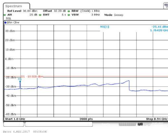
Figure 443 Spurious Emissions (1 GHz – 8.94 GHz) – 16QAM (876.5 MHz, 886.5 MHz 2 X 5 MHz Channel BW)
