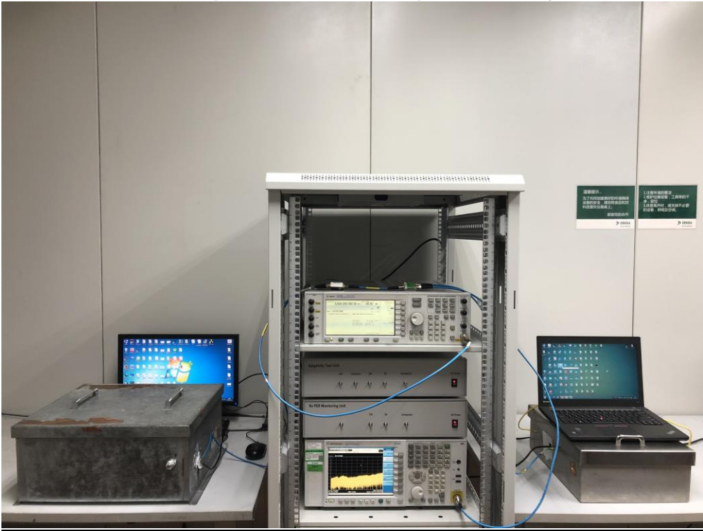
DFS Set-up Photo: Slave and Spectrum Analyzer
