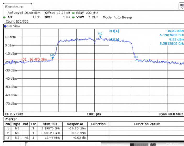
Fig. 2 Occupied 26dB Bandwidth (802.11a, 5200MHz)
