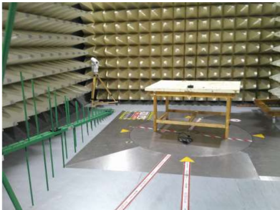
Photograph 2: Set-up for measurement of radiated emission
