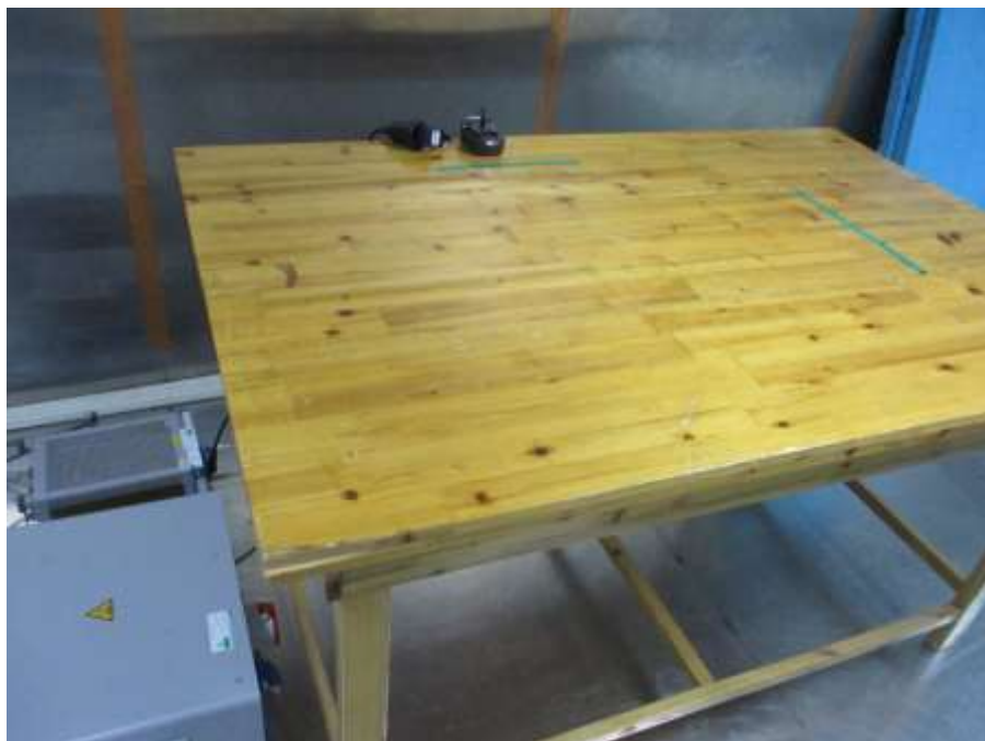
Photograph 2: Set-up for measurement of radiated emission
