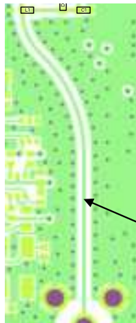
Figure 38: 50 \Omega grounded coplanar waveguide transmission line designed on the u-blox host PCB bottom layer
