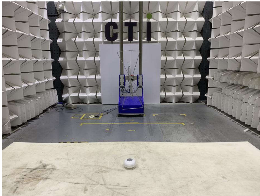
Radiated spurious emission Test Setup-1(Below 1GHz)
