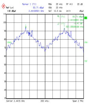
GN Mobile EUT: HS-73W. FCC Part 15.247 Carrier Separation Comment A: 48335JD08 Tx Mode, Hopping on All Channels, GFSK Mod. Date: 30.JUN.2006 12:18:16
