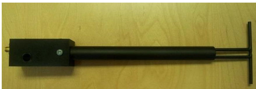
Figure 1 – MVG COMOSAR Validation Dipole
