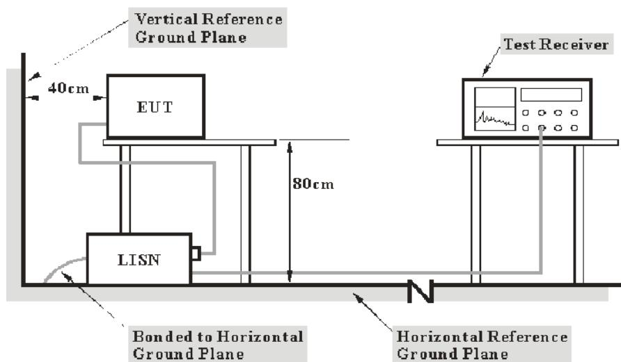
The measurement procedure of EUT setup is according with ANSI C63.10-2013. The related limit was specified in FCC Part 15.207.
