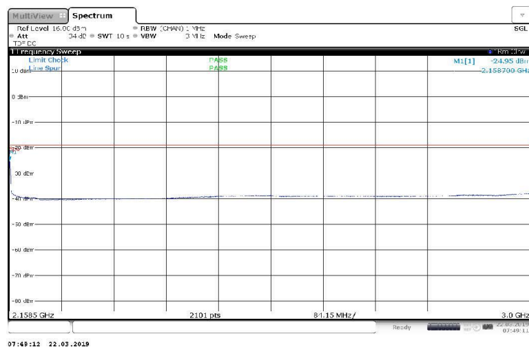
Figure 34 Spurious Emissions (2.1585 GHz – 3 GHz) – 16QAM (2155 MHz, 5 MHz Channel BW)
