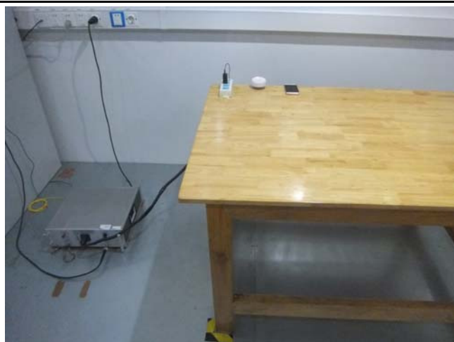
Conducted Emissions Test Setup – Front View
