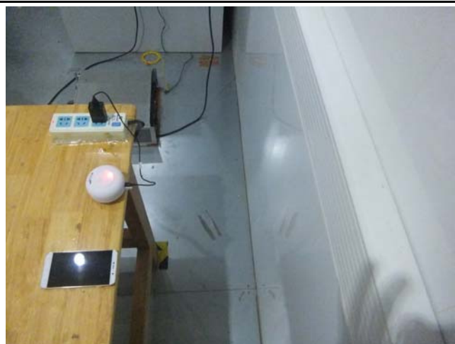
Conducted Emissions Test Setup – Side View
