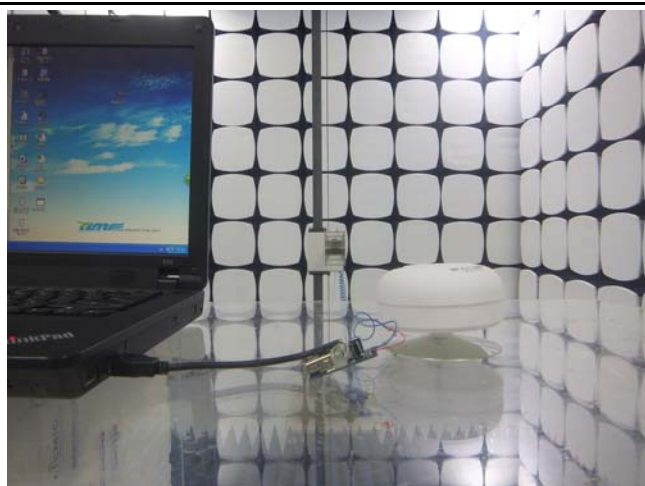
Radiated Spurious Emissions Test Above 1GHz
