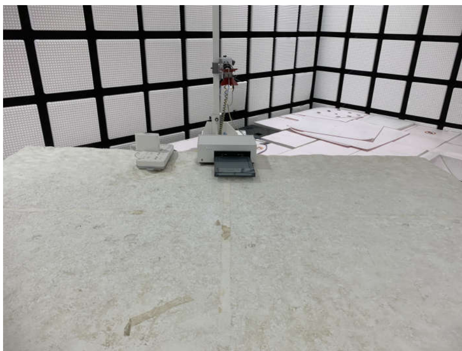
Radiated spurious emission Test Setup-2(Above 1GHz)
