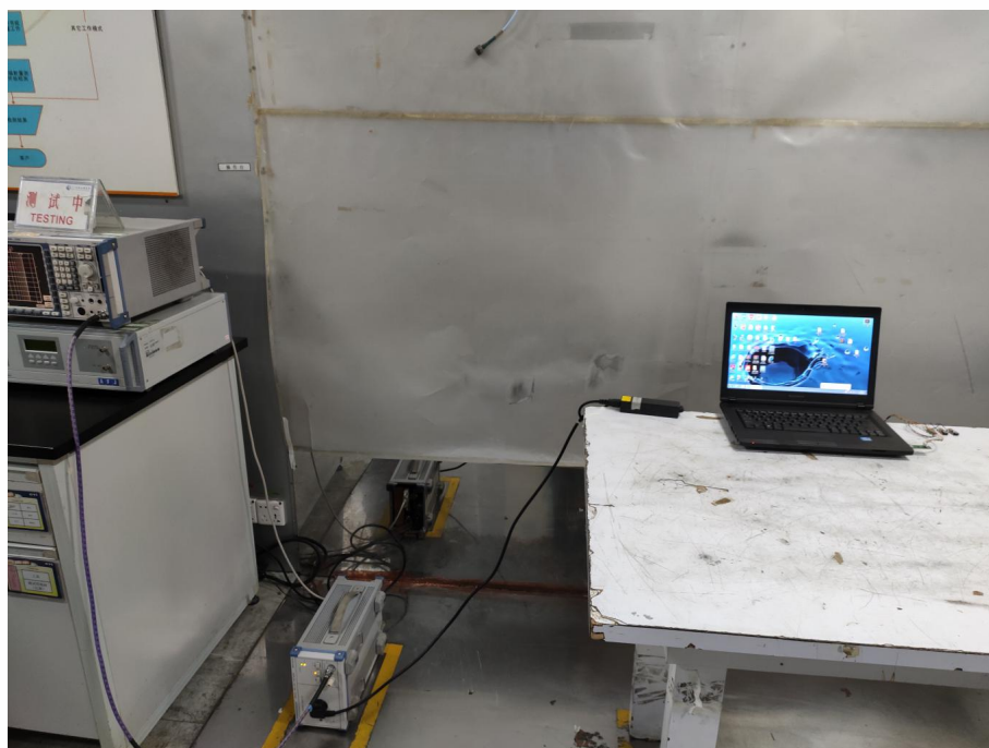
Conducted Emissions Test Setup
