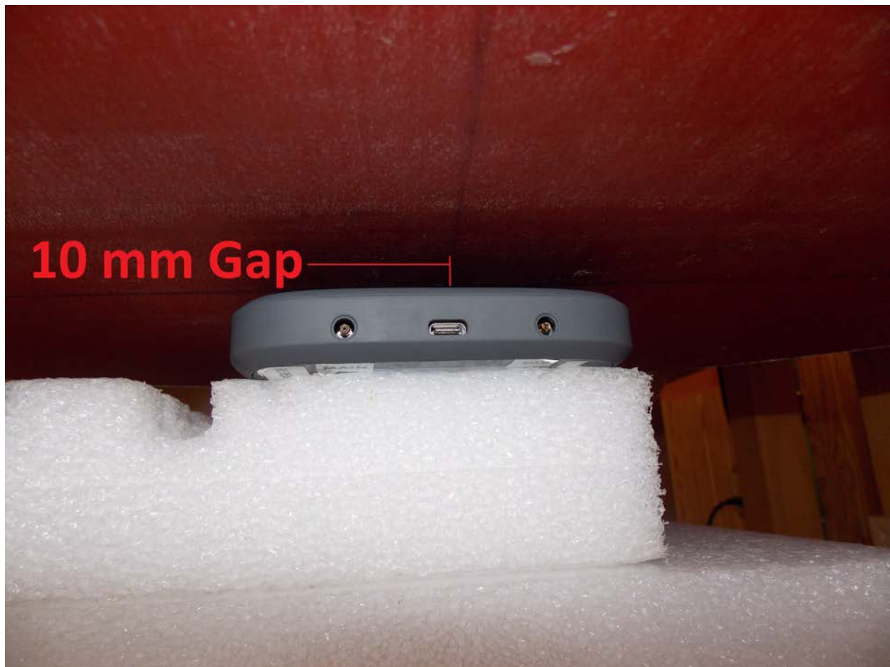
Test Position Side C 10 mm Gap
