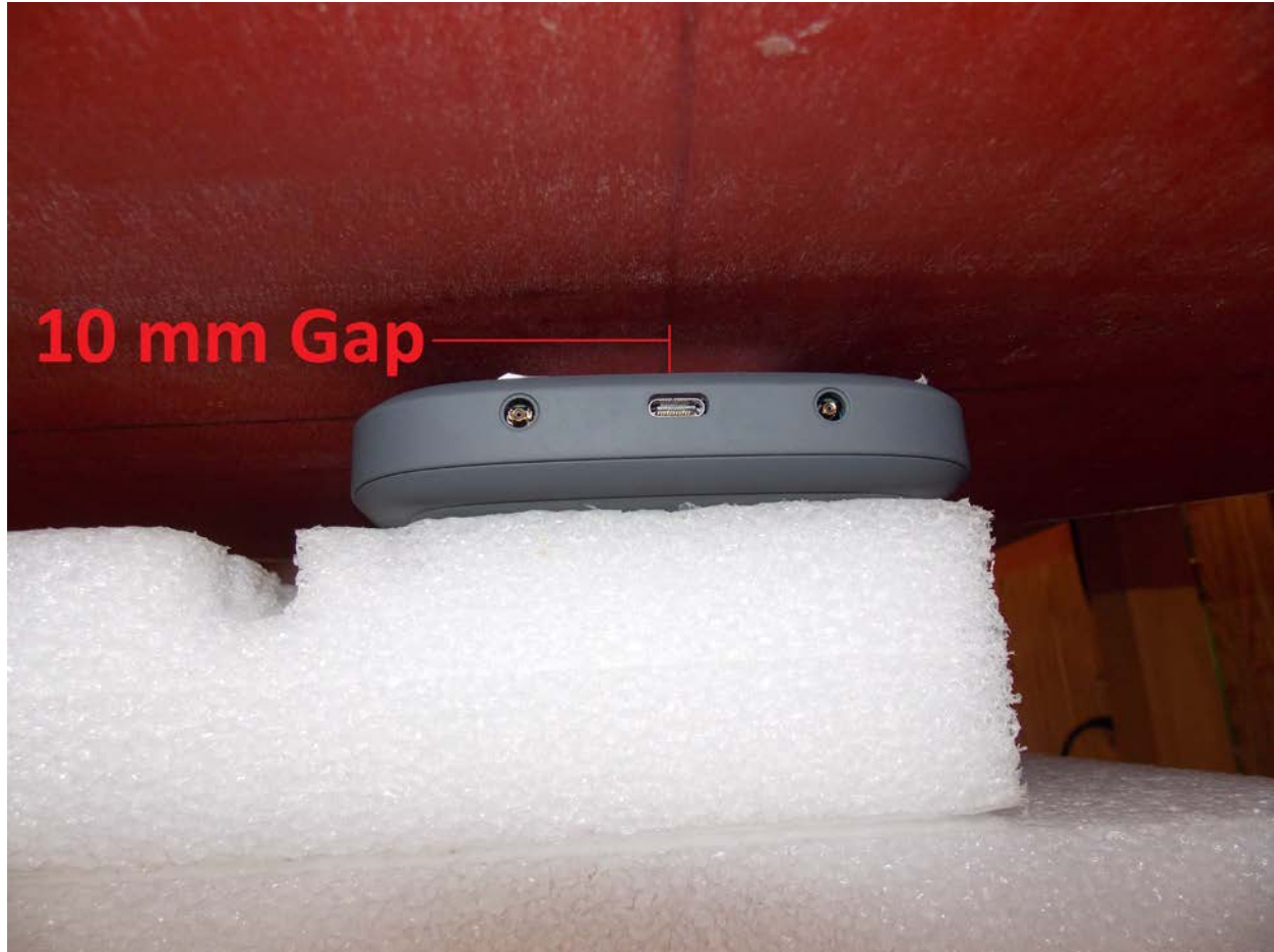
Test Position Side A 10 mm Gap
