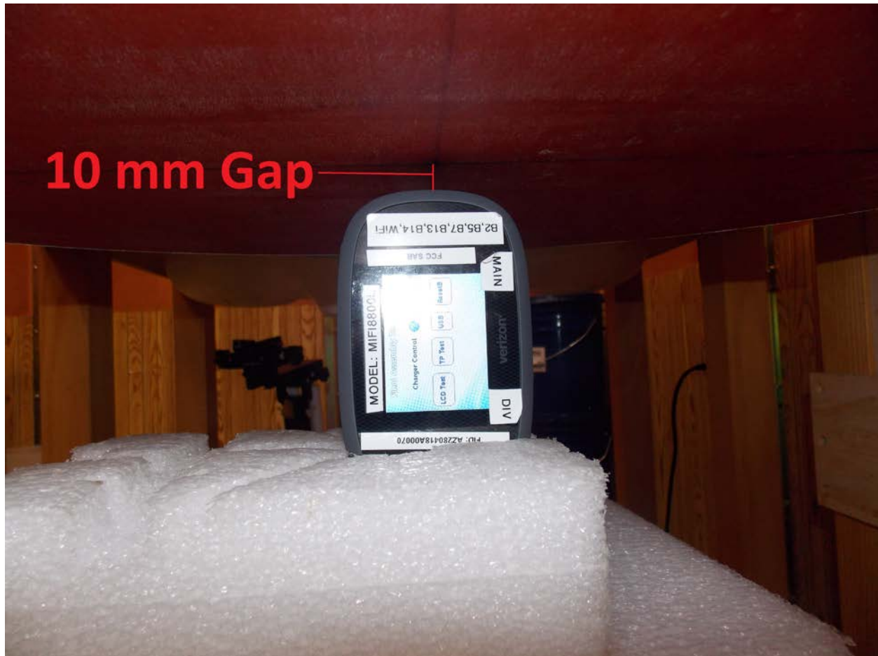
Test Position Side E 10 mm Gap
