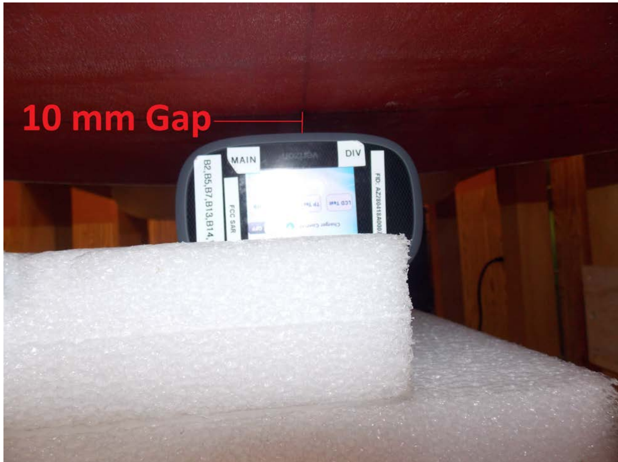
Test Position Side B 10 mm Gap
