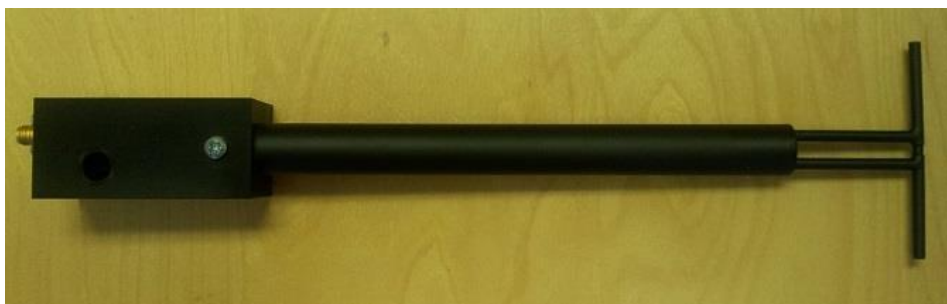
Figure 1 – MVG COMOSAR Validation Dipole
