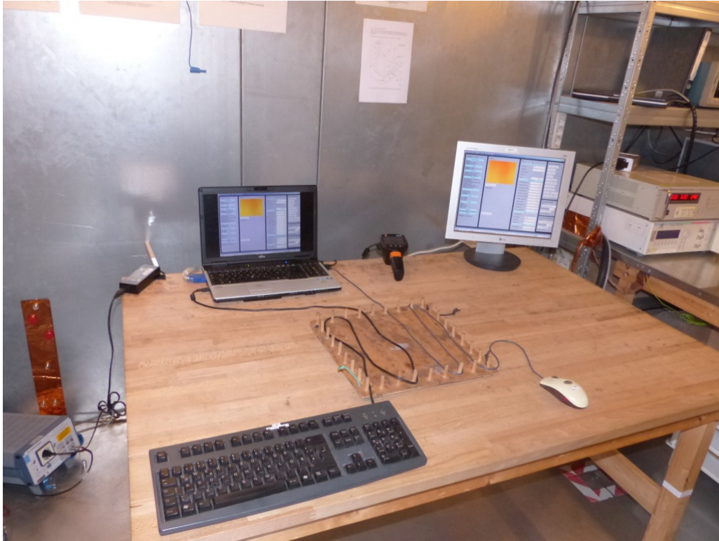
Photo 3: Test setup for conducted measurements (AC/DC adapter, 120 V/60 Hz, EMC insulated room, unintentional radiator, § 15)
