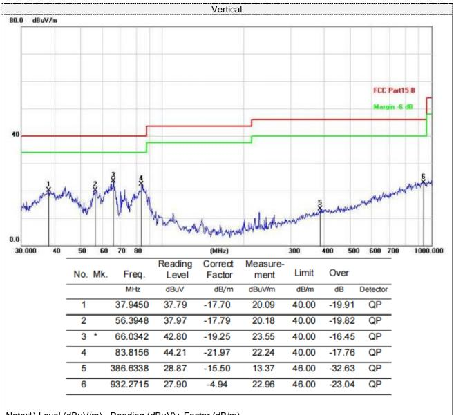
Note:1).Level  $(dB\mu V/m)$ = Reading  $(dB\mu V)$ + Factor (dB/m)
