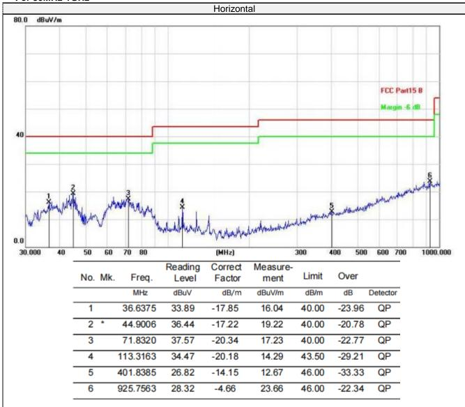
Note:1).Level ( $dB\mu V/m$ )= Reading ( $dB\mu V$ )+ Factor (dB/m)
