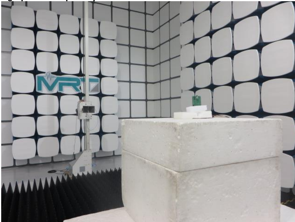
Photograph 3: Set-up for Spurious Emissions above 1GHz
