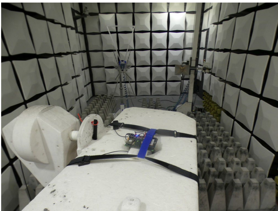
Photo 3: Test Antenna for radiated measurements above 1GHz
