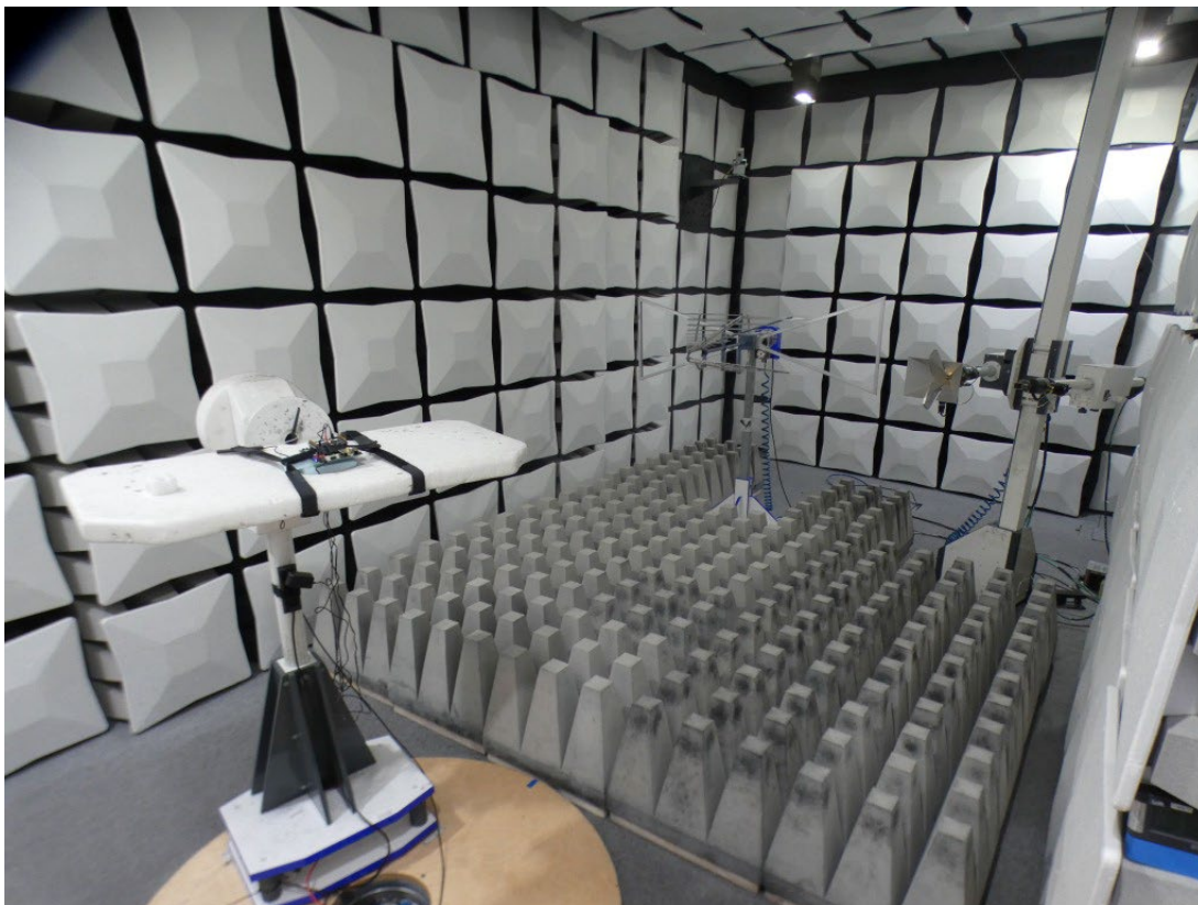
Photo 1: Test setup for radiated measurements above 1GHz
