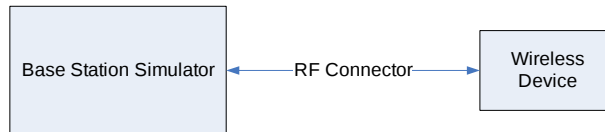
Figure 9-3 Power Measurement Setup
