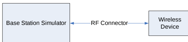
Figure 9-1 Power Measurement Setup
