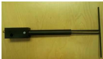
Figure 1 – MVG COMOSAR Validation Dipole
