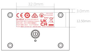
Label: Due to the size, appearance, shape, cost and shell material of the product, the warning words related to the requirements of FCC Part 15.19 cannot be placed on the product mainbody, thus the content of the warning words will be described in the user manual.
