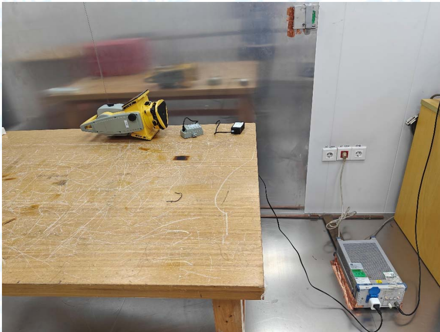
Photo of Setup for Conducted Emission
