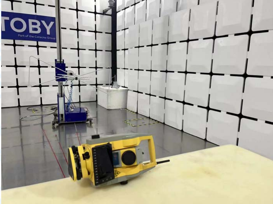
Photo of Setup for Radiated Emission (30MHz~1GHz)
