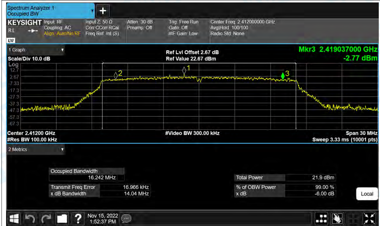
-6dB Bandwidth NVNT g 2412MHz Ant1
