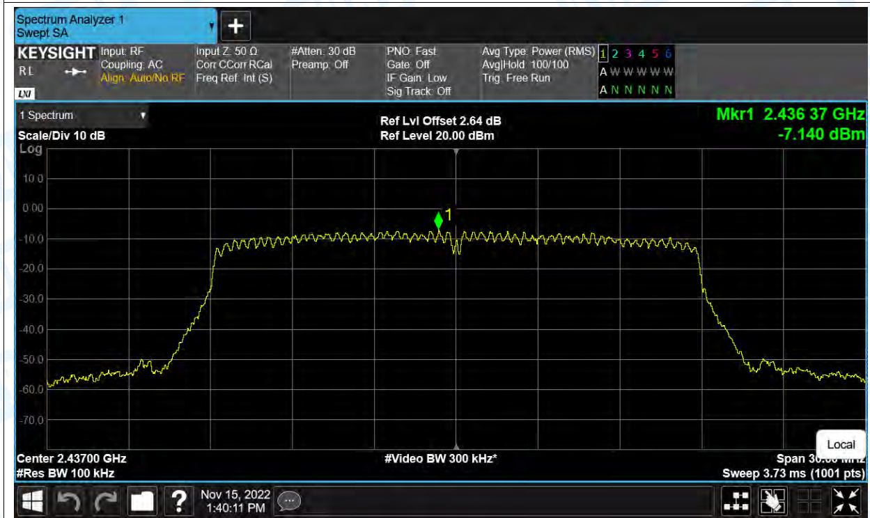
PSD NVNT n(HT20) 2437MHz Ant1
