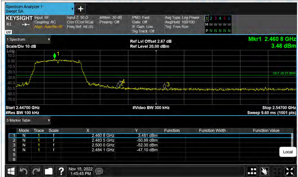
Band Edge NVNT g 2462MHz Ant1 Emission
