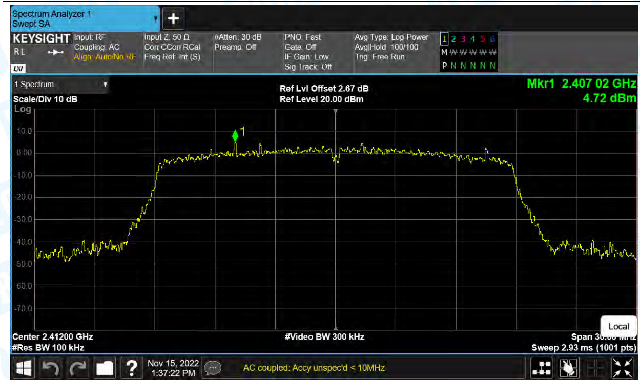
Band Edge NVNT n(HT20) 2412MHz Ant1 Emission
