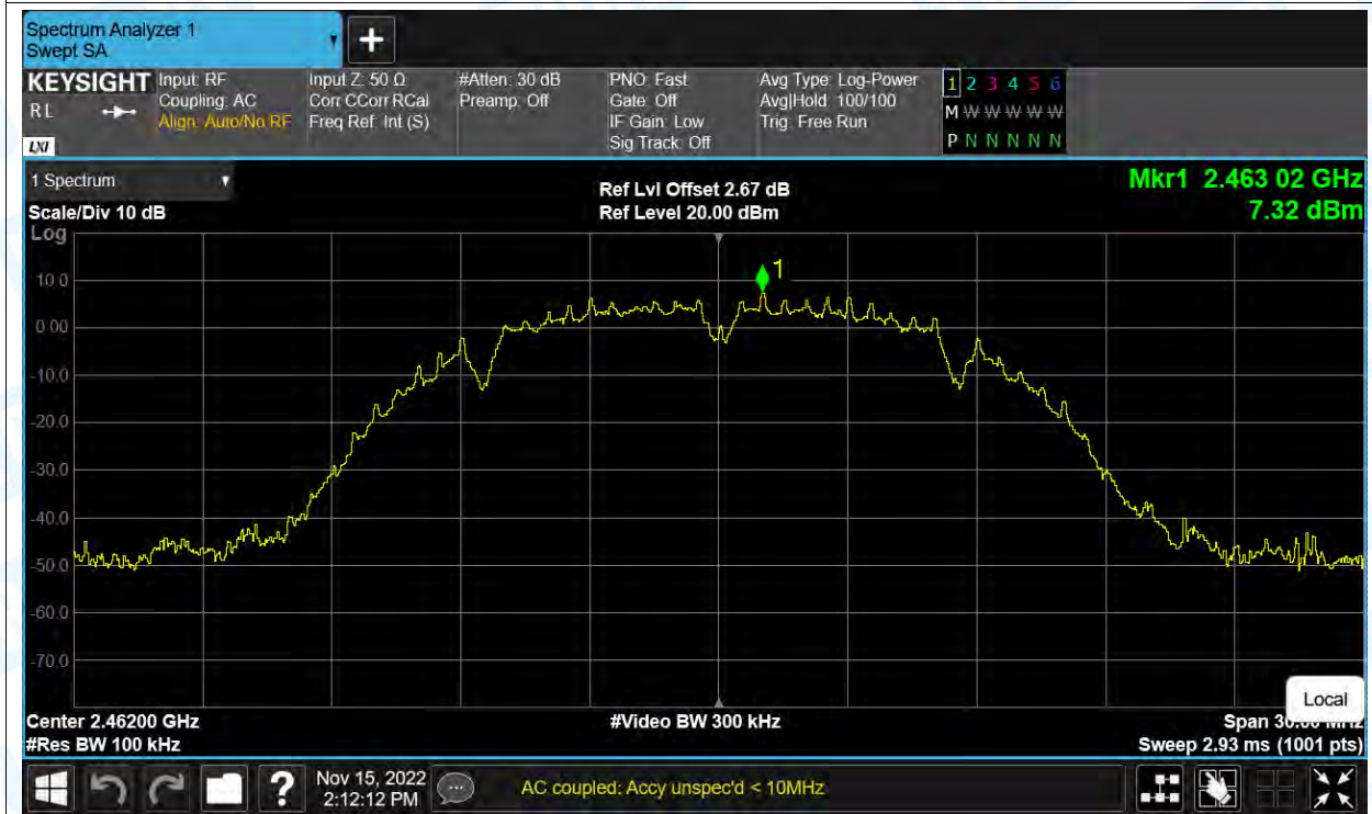
Tx. Spurious NVNT b 2462MHz Ant1 Emission
