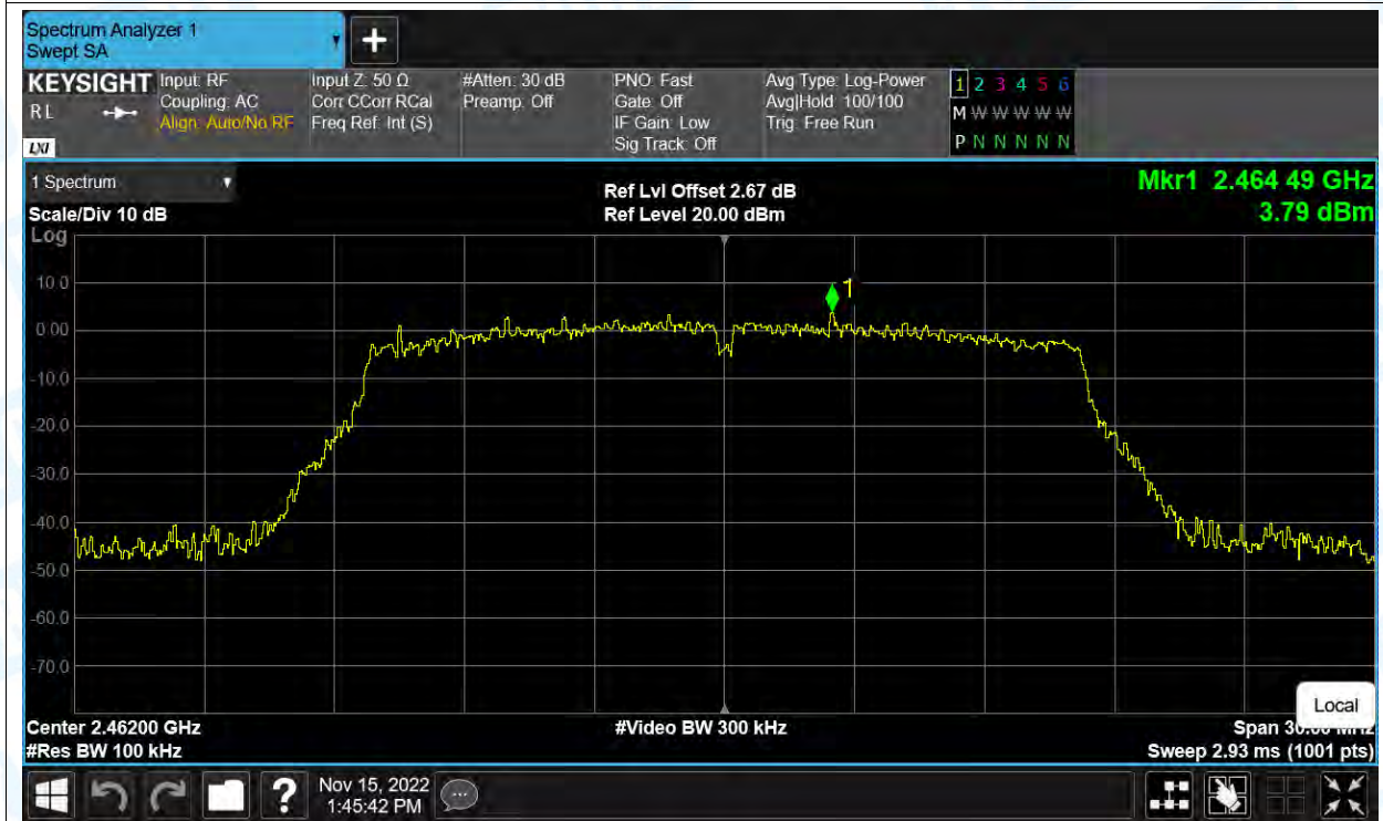
Band Edge NVNT g 2462MHz Ant1 Emission
