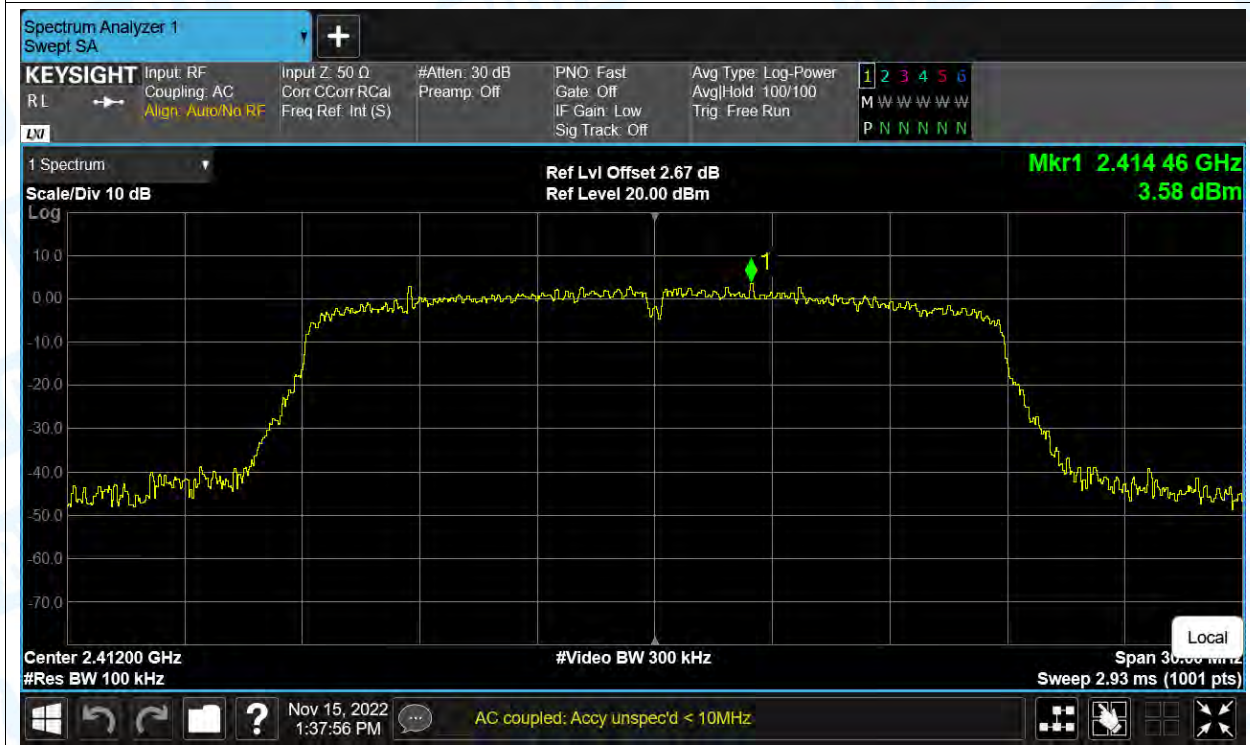
Tx. Spurious NVNT n(HT20) 2412MHz Ant1 Emission
