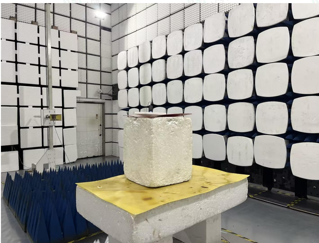
Radiated Emissions Measurement (Above 1GHz)
