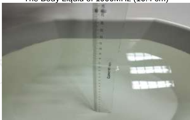
The Body Liquid of 2600MHz (16.5cm)
