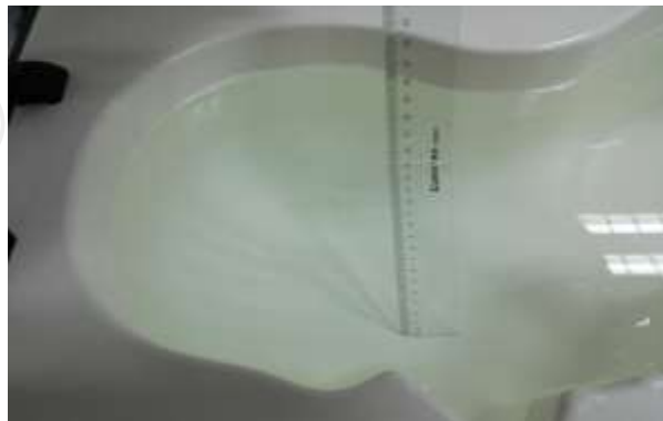
The Head Liquid of 1800MHz (15.2cm)
