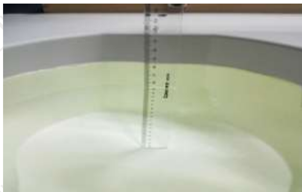
The Body Liquid of 1800MHz (15.2 cm)
