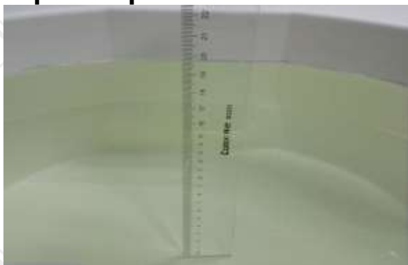
The Body Liquid of 835MHz (15.4cm)
