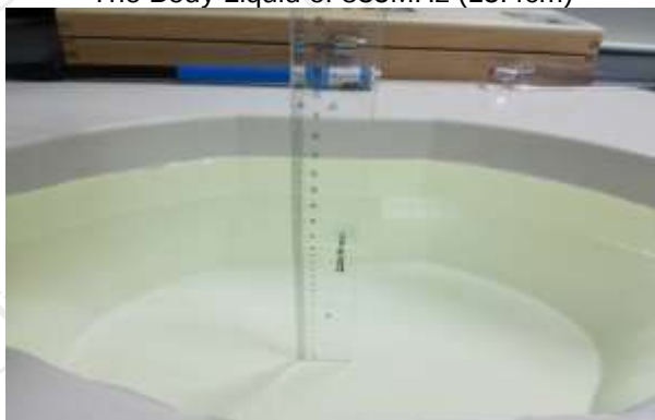
The Body Liquid of 1900MHz (16.4 cm)
