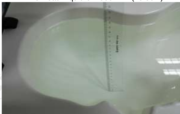
The Head Liquid of 2600MHz (15.1cm)
