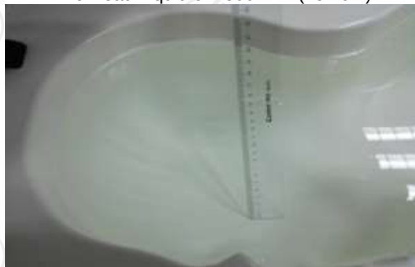
The Head Liquid of 2450MHz (15.6cm)
