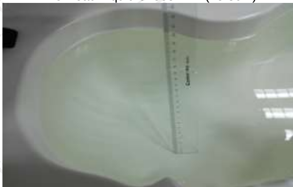
The Head Liquid of 1900MHz (15.5cm)
