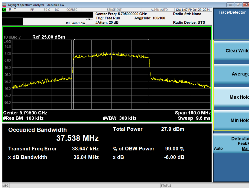
Plot 7-8. 6dB BW & 99% OBW Antenna WF7a (40MHz BW 802.11ax (SU) – Ch. 159)
