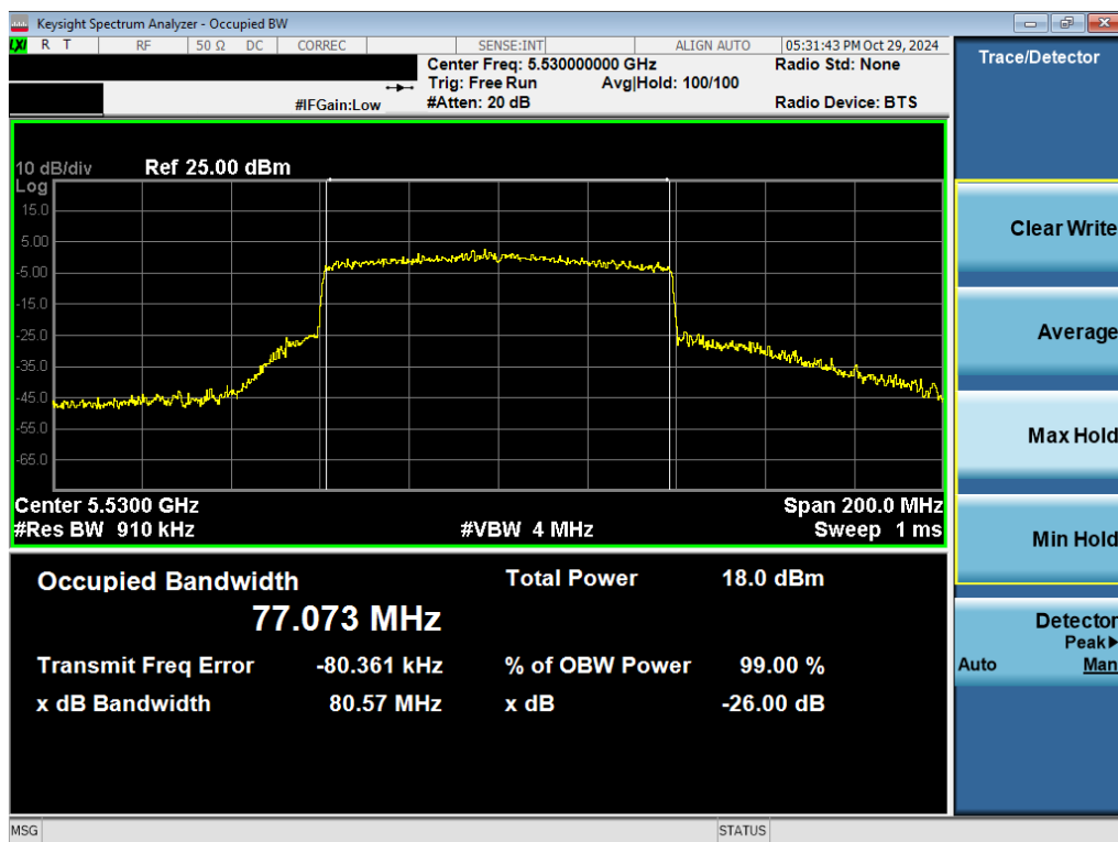
Plot 7-6. 26dB BW & 99% OBW Antenna WF8 (80MHz BW 802.11ax(SU) – Ch. 106)
