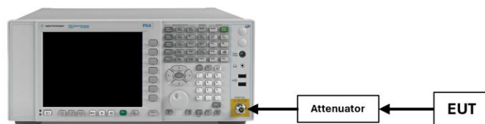
Figure 7-1. Test Instrument & Measurement Setup
