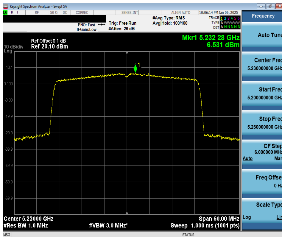
Plot 7-23. PSD Antenna WF8 (40MHz BW 802.11ax SU – Ch. 46)
