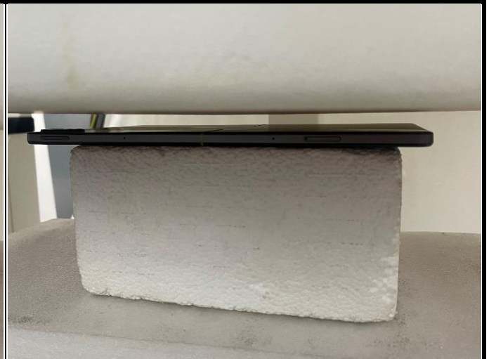
Rear Face of EUT with 1.0 cm Gap
