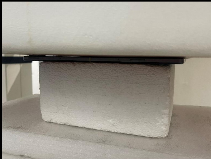
Rear Face of EUT with 0 cm Gap
