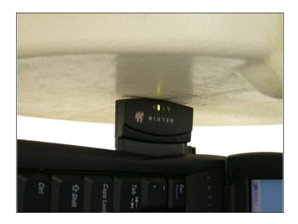
**EUT** to the phantom distance 0mm
