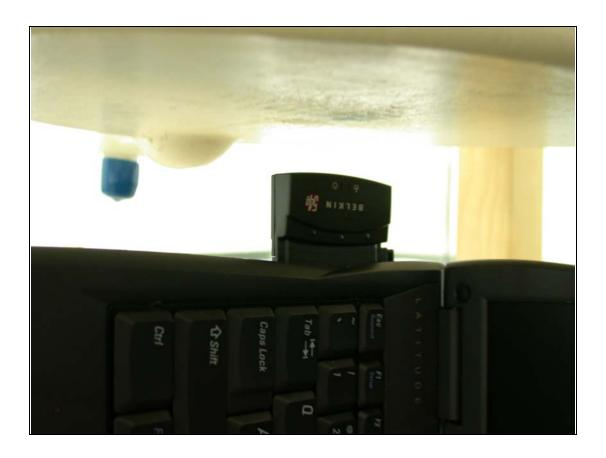
**EUT** to the phantom distance 15mm
