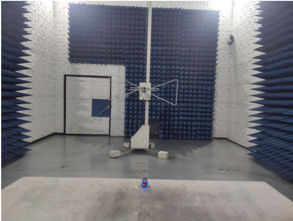
RADIATED EMISSION TEST SETUP ABOVE 1GHz
