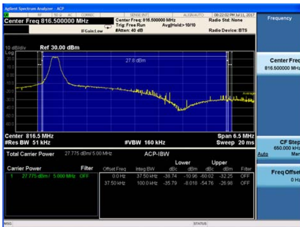
LTE Band 26 QPSK 1RB CH Low 5M
