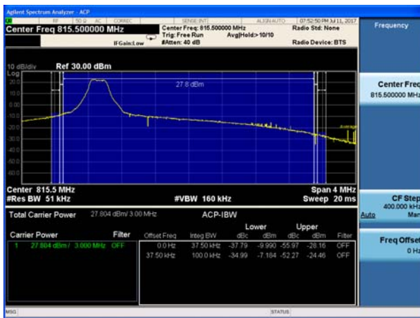
LTE Band 26 QPSK 1RB CH Low 5M
