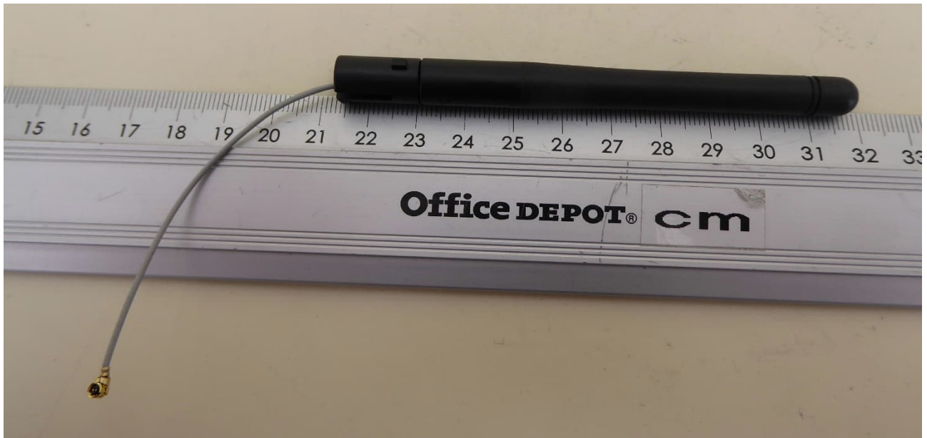
Monopole ( \frac{1}{4} wave) antenna W1039B030 by Pulse Electronic / Yageo
