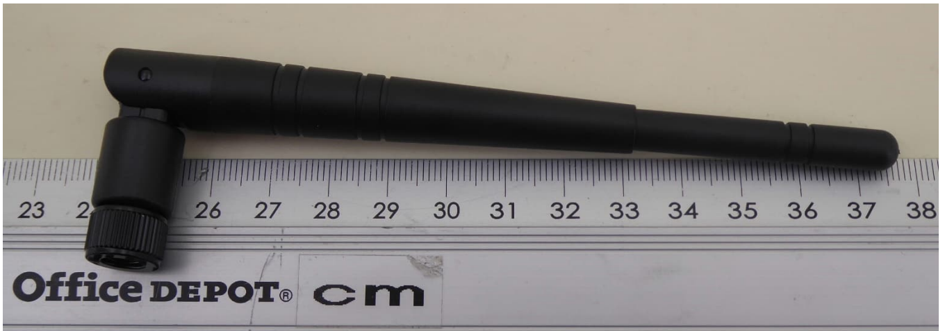
Monopole ( \frac{1}{2} wave) antenna GW.59.3153 by taoglas
