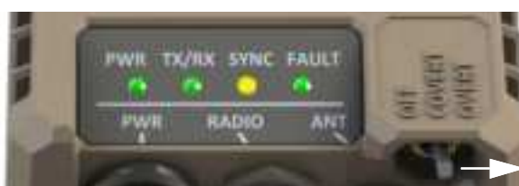
Figure 2-2: Synchronization process in LEDs
