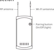
① The device weight is less than 1 kg. The installation height of less than 2 m is recommended.
