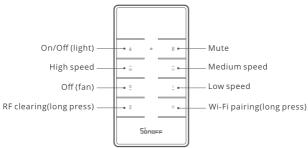
**RF clearing method:** Long press for 5s until the ceiling fan makes two sounds "di di" to clear the code successfully.
