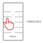
Please press any button within 5s after powering on again untilthe ceiling fan makes a sound "di", and pairing is successful.
