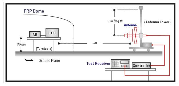
Above 1GHz Test Setup:
