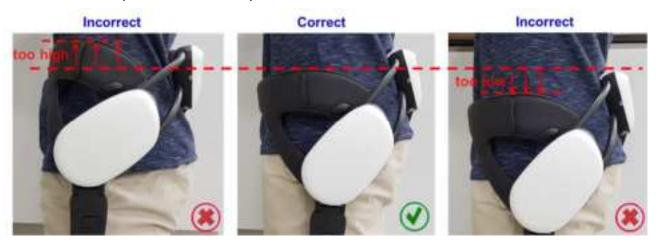
2) Examples of correct and incorrect thigh support frame positioning:
