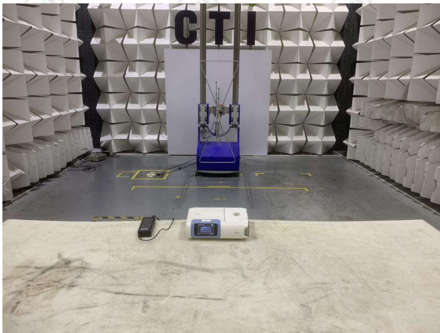
Radiated spurious emission Test Setup-1(Below 1GHz)
