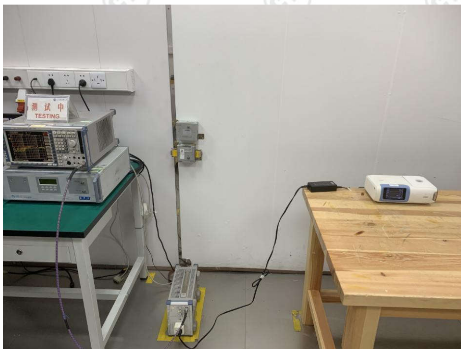
Conducted Emissions Test Setup
