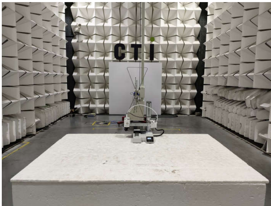
Radiated spurious emission Test Setup-1(Below 1GHz)
