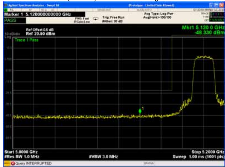
802.11ac(VHT20) U-NII-1 Band edge-left side
