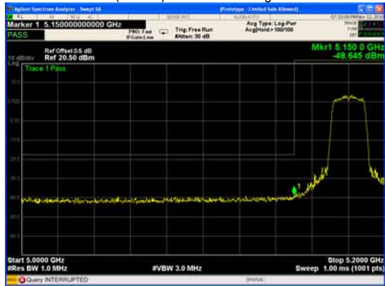
802.11ac(VHT20) U-NII-1 Band edge-left side
