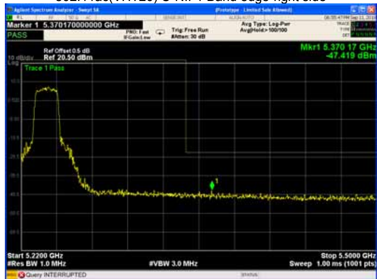
802.11ac(VHT20) U-NII-1 Band edge-right side
