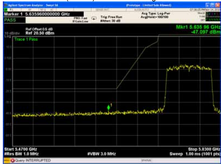
802.11ac(VHT80) U-NII-3 Band edge-left side
