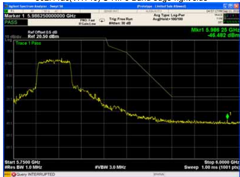
802.11ac(VHT40) U-NII-3 Band edge-right side
