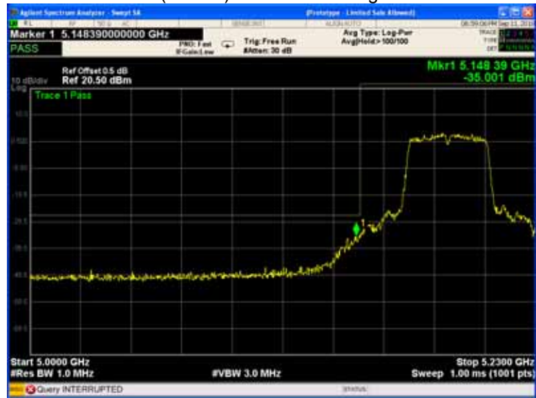
802.11ac(VHT40) U-NII-1 Band edge-left side
