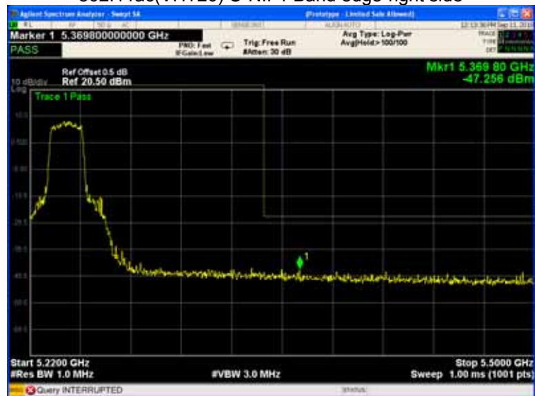
802.11ac(VHT20) U-NII-1 Band edge-right side
