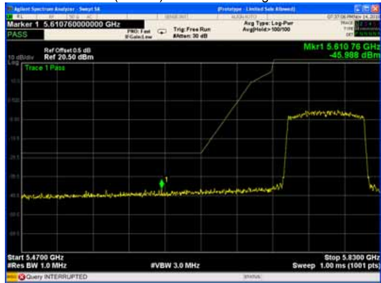
802.11ac(VHT80) U-NII-3 Band edge-left side
