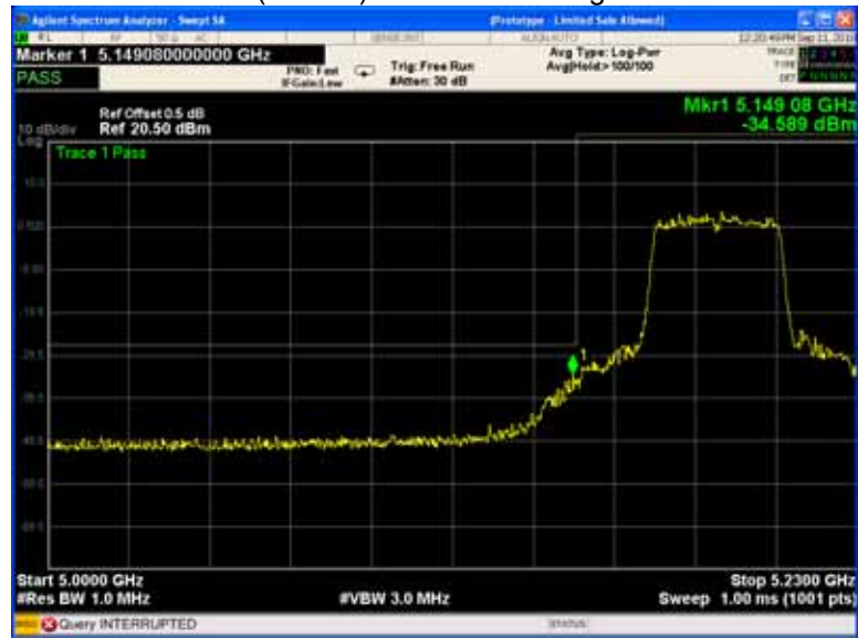
802.11ac(VHT40) U-NII-1 Band edge-left side
