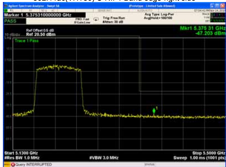
802.11ac(VHT80) U-NII-1 Band edge-right side
