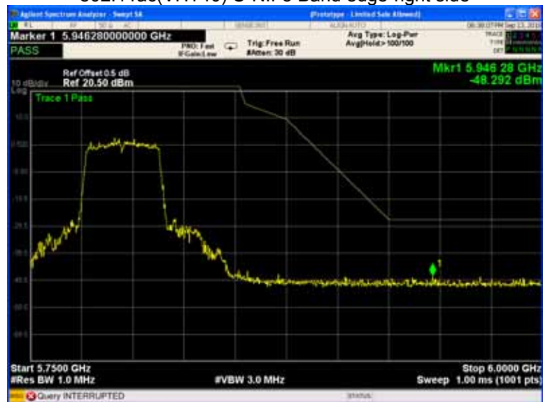
802.11ac(VHT40) U-NII-3 Band edge-right side
