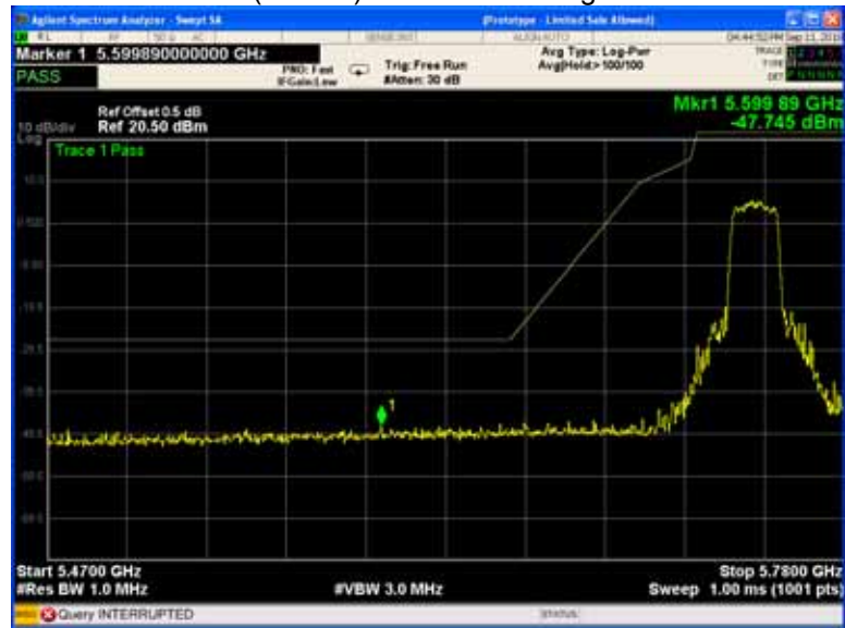
802.11ac(VHT20) U-NII-3 Band edge-left side
