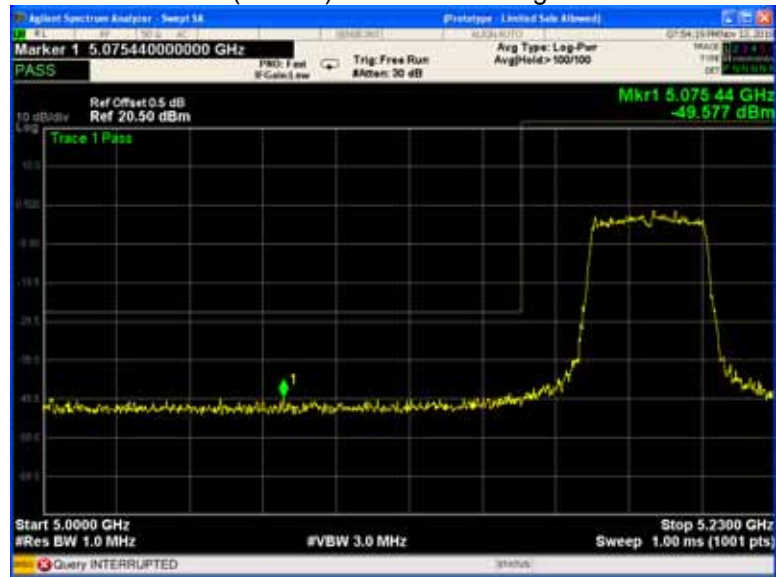
802.11ac(VHT40) U-NII-1 Band edge-left side
