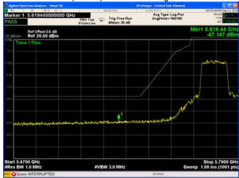
802.11ac(VHT40) U-NII-3 Band edge-left side
