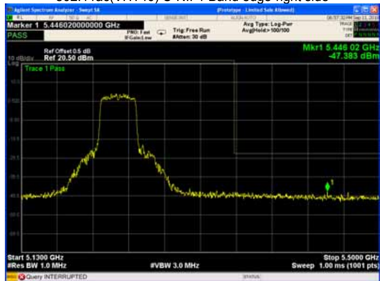
802.11ac(VHT40) U-NII-1 Band edge-right side
