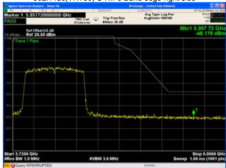
802.11ac(VHT80) U-NII-3 Band edge-right side
