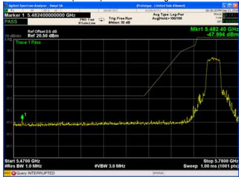
802.11ac(VHT20) U-NII-3 Band edge-left side
