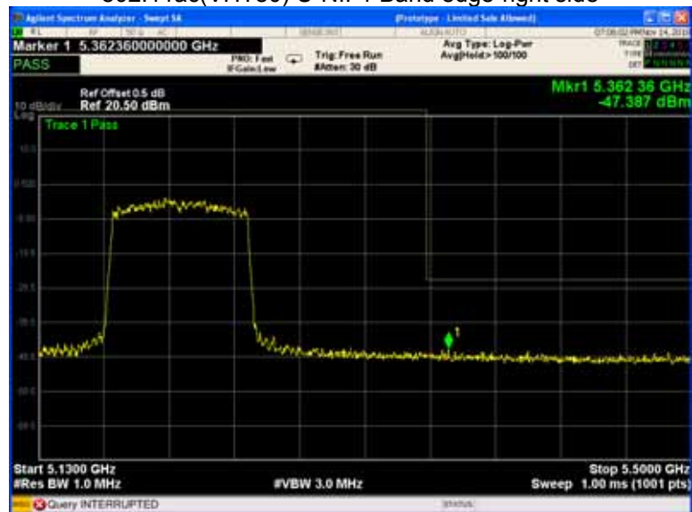
802.11ac(VHT80) U-NII-1 Band edge-right side
