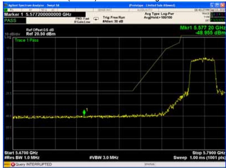
802.11ac(VHT40) U-NII-3 Band edge-left side
