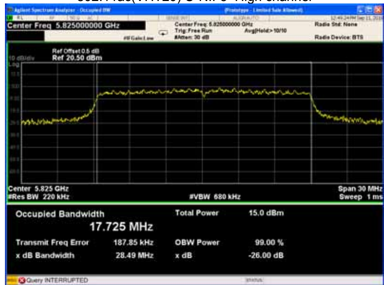
802.11ac(VHT20) U-NII-3 High channel
