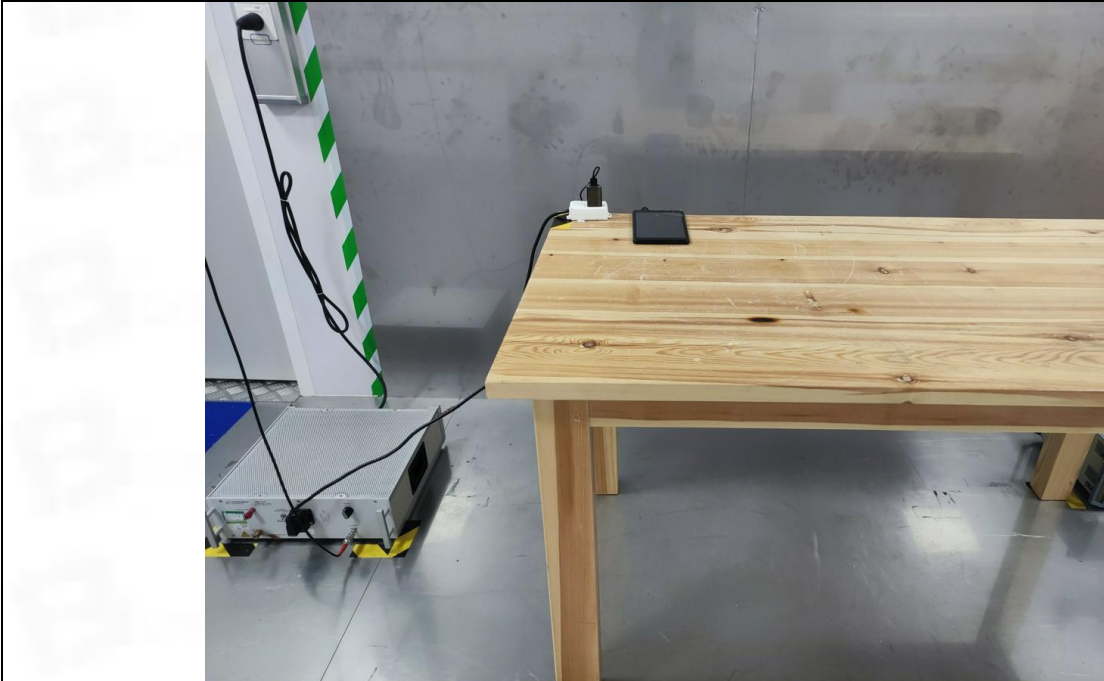
Conducted Emission at AC power line
