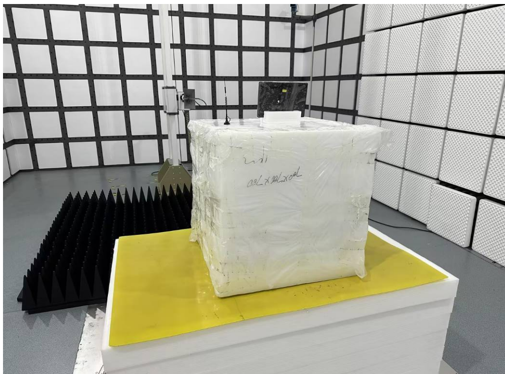
Photo of Radiated Emission Measurement (Above 1G)
