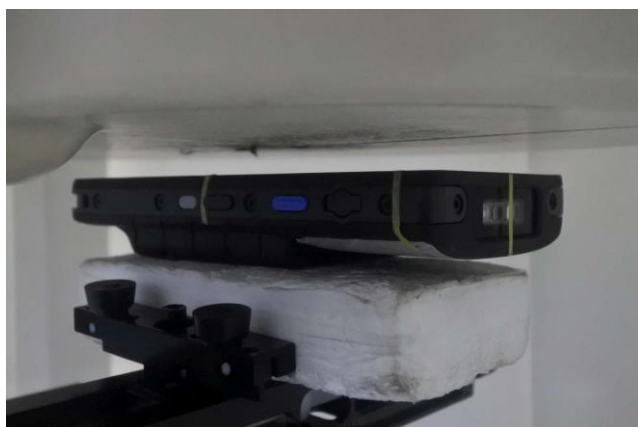
Front, Test Separation 10 mm for Battery2&3
