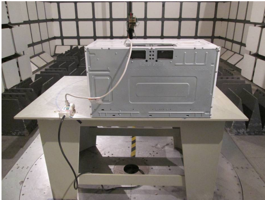
Radiated Emissions - Rear View (Above 1 GHz)
