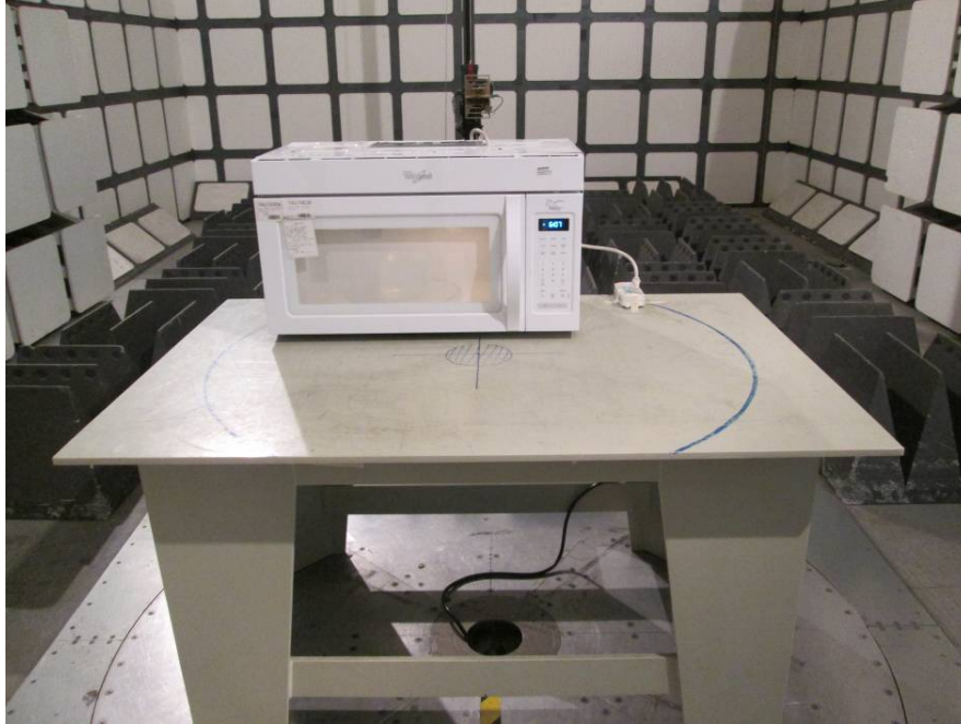
Radiated Emissions - Front View (Above 1 GHz)
