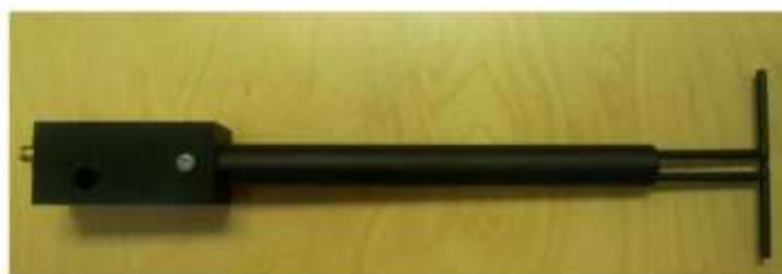
Figure 1 – MVG COMOSAR Validation Dipole
