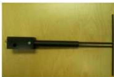
Figure 1 – MVG COMOSAR Validation Dipole
