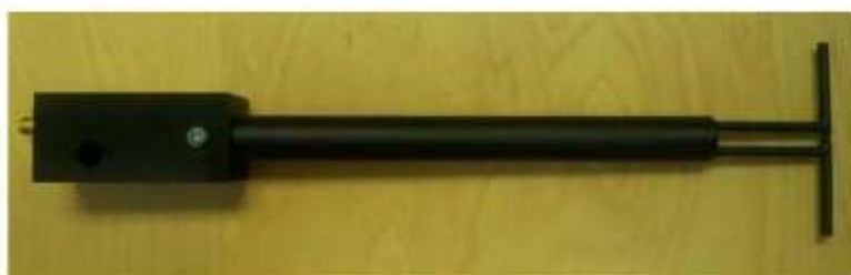
Figure 1 – MVG COMOSAR Validation Dipole
