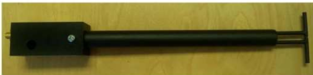
Figure 1 – MVG COMOSAR Validation Dipole
