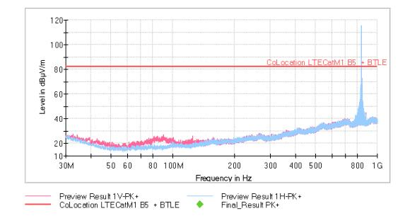
The peak above the limit is the Carrier frequency LTE Band 5 (836.5 MHz).
