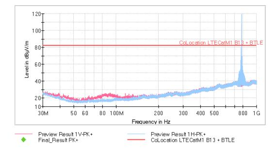
The peak above the limit is the Carrier frequency LTE Band 13 (782.0 MHz).
