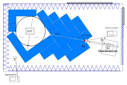
Radiated measurements above 17 GHz.
