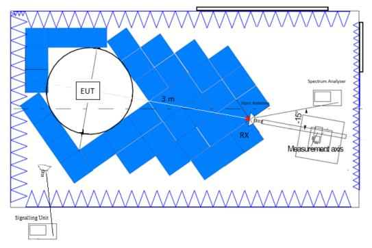
Radiated measurements above 17 GHz.
