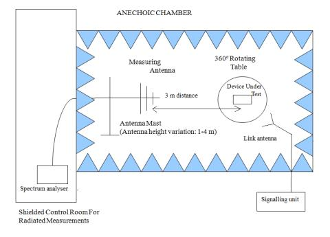
Radiated measurements setup between 1 GHz to 17 GHz.
