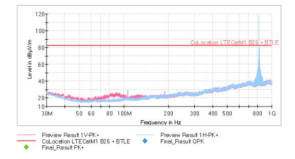
The peak above the limit is the Carrier frequency LTE Band 26 (819.0 MHz).
