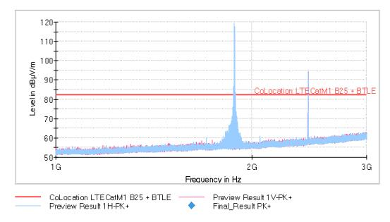
The peak above the limit on the left is the Carrier frequency LTE Band 25 (1882.5 MHz). The peak above the limit on the right is the Carrier frequency Bluetooth Low Energy (2440 MHz).
