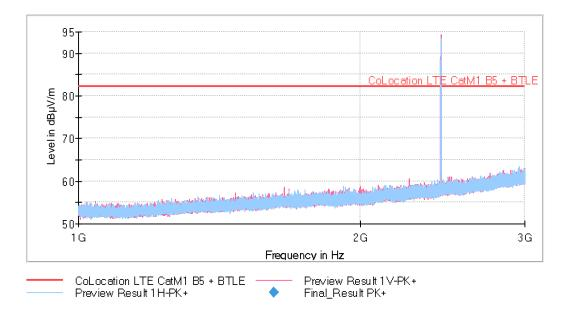
The peak above the limit is the Carrier frequency Bluetooth Low Energy (2440 MHz).
