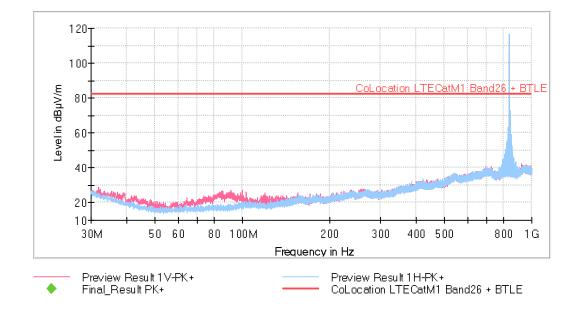
The peak above the limit is the Carrier frequency LTE Band 26 (836.5 MHz).
