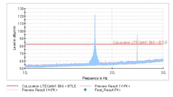
The peak above the limit on the left is the Carrier frequency LTE Band 66 (1745.0 MHz). The peak above the limit on the right is the Carrier frequency Bluetooth Low Energy (2440 MHz).
