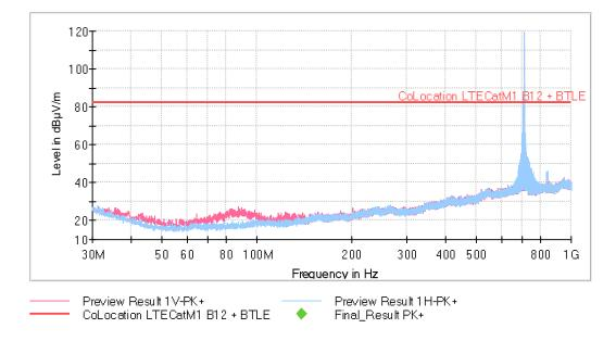
The peak above the limit is the Carrier frequency LTE Band 12 (707.5 MHz)
