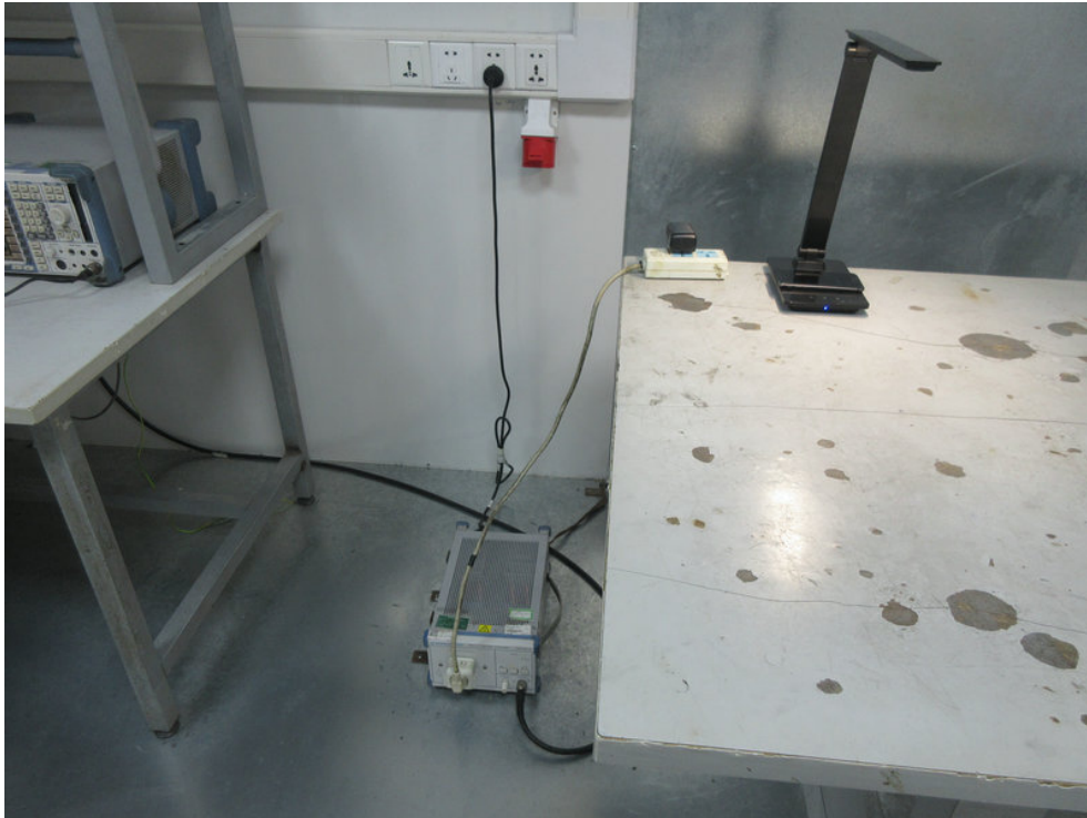
Photo of Conducted Emission Measurement
