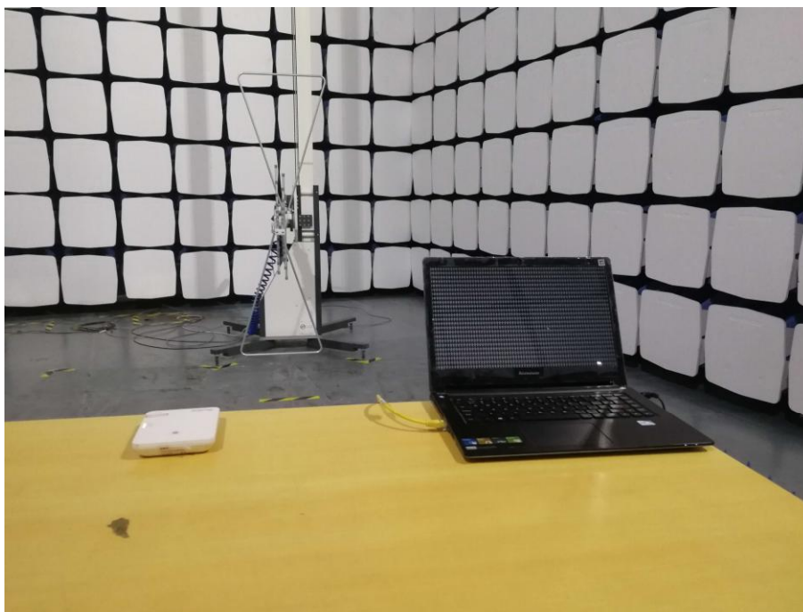
FP - Radiated Emission test view (Frequency from 30MHz to 1GHz)
